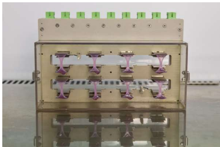
Figure 1. Equivalent dermis in GlasBox Plus ® device. This patented device could measure the contractile forces of the human primary fibroblasts through 2 thin electrodes in each well. The distance between the 2 plates which demonstrates the force, could be measured automatically by the device software.
